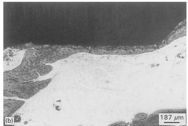
Figure 4 Light micrograph of (a) an HA-PS coated implant, and (b) a FA/HA-PS coated implant, both after 6 months of implantation. Good bone implant contact can be observed.
